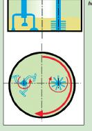
horizontal since 1924. R type mixer, rotating pan, inclined since 1970.
