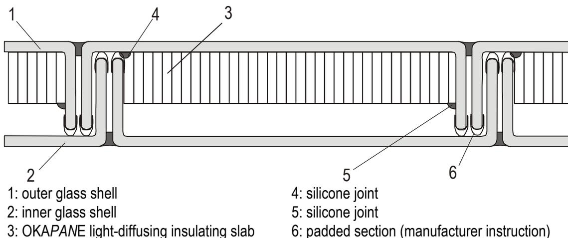
The width recommendations are non-binding and must be checked by the glazier. If other widths are necessary because the joint distances are different or a padded profile is being used, this must be noted down on the order. If a padded section is used the above mentioned OKAPANE with ha to be reduced by 2 mm. We recommend using a padded section without protruding lips since these can lead to problems during assembly.
