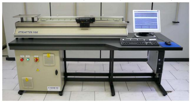
Striagraph model Striatter 1000™ is a modern machine that creates image of striaes, bubbles and other non-homogeneities in thickness of sheet glass. Such an image is called a striagram and its practical use is quality measuring of examined sample of glass.
