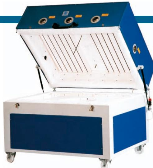
Kiln for the production of transparent washbasins which can be equipped with one, two or four holes for the production of one or more single/double basins.
