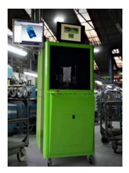
ariScann aims to provide automatic mould scanning and measuring. The device provides highly accurate 3D scanning, along with a specifically developed software that allows automatic dimensional control of moulds.
