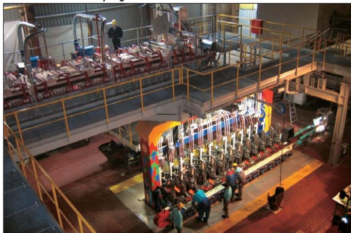
▼ NIS 5" triple gob 10 Section: servo mould open and close and servo FlexIS Pusher.
