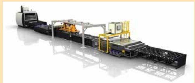
This system is the only one in the world that has three lamination phases in independent chambers, which gives the professional great flexibility. It has been designed to extract moisture from the interlayer without the need to use traditional autoclave systems, for which energy efficiency costs are drastically reduced. Pujol 100 PVB+ is considered to be an ideal solution for glass transformers with productions of between 5,000 and 15,000 m<sup>2</sup> per month.
