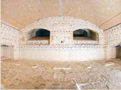
**The new end fired furnace, which produces container glass in the colours amber and green, was finally successfully commissioned at the end of the first quarter of 2022**
