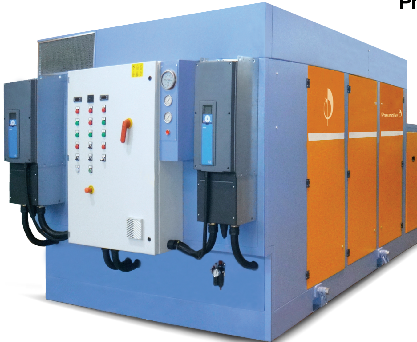
UV100 VS220 HC - 1890 to 6480 m 3 /h, 2 x 110kW air cooled for hot climate, lubricated, rotary vane, single stage vacuum pump
