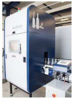
The Separator allows bottles and/or jars to be distributed between up to four tracks without changing the production speed. With its fast industrial image processing in combination with the corresponding SPS-programming, Bertram's system works so flexibly that it can handle all standard tasks. Resulting, in essence, from the shape and number of bottles and/ or jars, and their allocation to the correct tracks.
